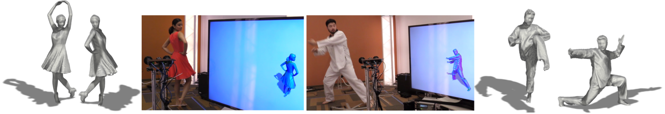
Figure 1: We present a new method for real-time high quality 4D (i.e. spatio-temporally coherent) performance capture, allowing for incremental nonrigid reconstruction from noisy input from multiple RGBD cameras. Our system demonstrates unprecedented reconstructions of challenging nonrigid sequences, at real-time rates, including robust handling of large frame-to-frame motions and topology changes.
