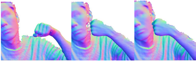
Figure 5: Left: reference surface. Middle and Right: surfaces from warped volume without and with voxel collision detection.
