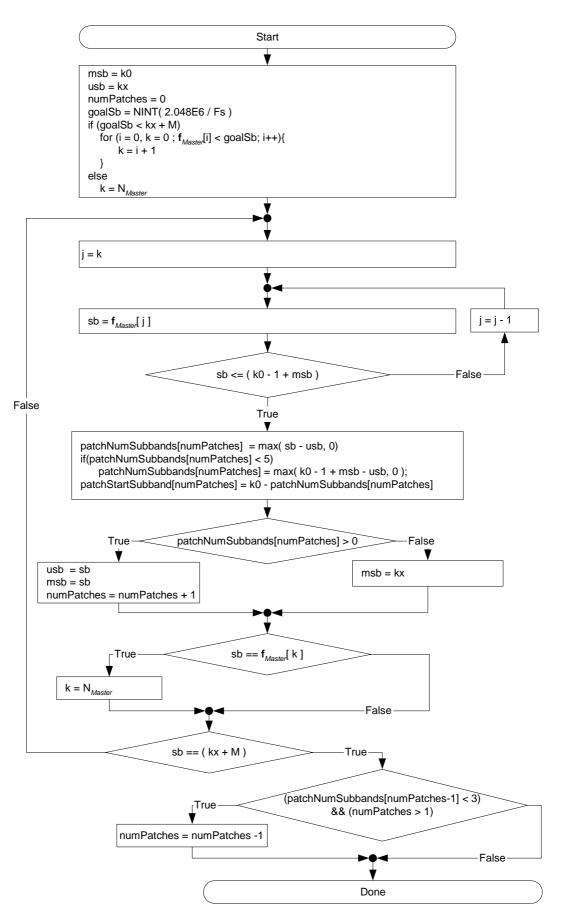
Figure 17: Flowchart of patch construction
