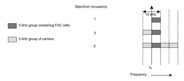
Figure 41: Spectrum occupancy for 10 kHz channels
