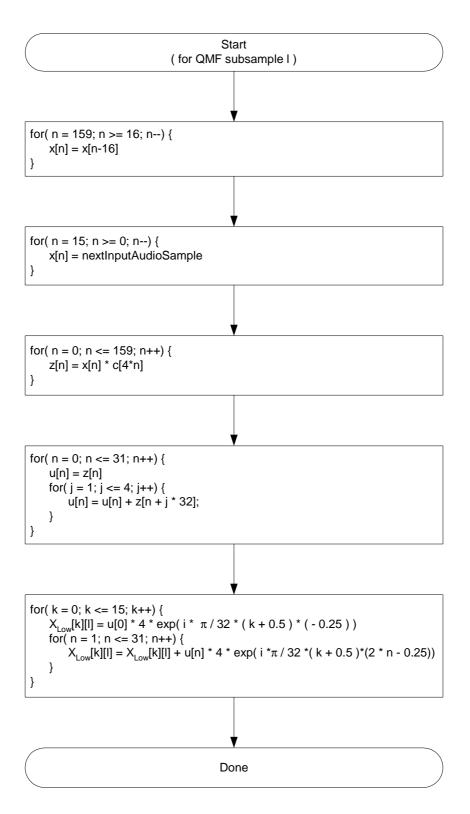
Figure 16: Flowchart of decoder 16-channel analysis QMF bank
