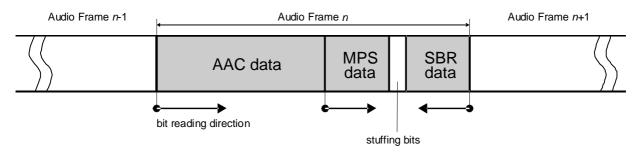
Figure 7: AAC + SBR + MPS frame
