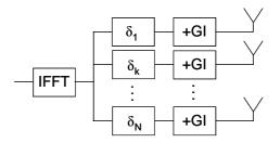
Figure P.1: Transmit delay diversity scheme
