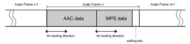
Figure 6: AAC + MPS frame
