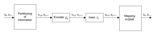
Figure 33: Multilevel coding with 1 level (SM)
