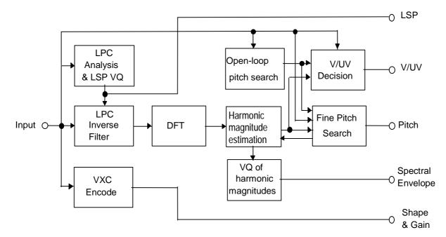
Figure 11: Block diagram of the HVXC encoder
