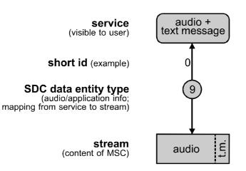
EXAMPLE 2: There are two audio services. Both point to the same audio stream. One of these services points to an additional packet mode data sub-stream carrying a multimedia data application. In total there are one audio stream and one data stream using packet mode.
