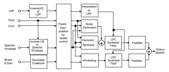
Figure 10: Block diagram of the HVXC decoder
