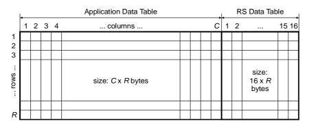
Figure 22: Structure of the FEC frame
