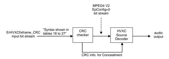
Figure 12: Block diagram of HVXC syntax
