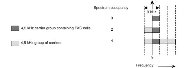
Figure 40: Spectrum occupancy for 9 kHz channels
