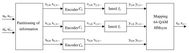
Figure 30: Multilevel coding with 3 levels for HMsym
