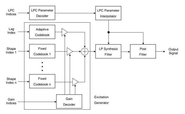
A basic block diagram of the CELP decoder is given in figure 8.
