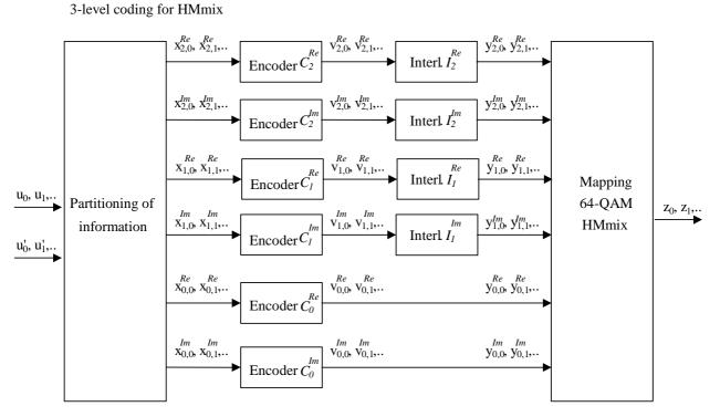
Figure 31: Multilevel coding with 3 levels for HMmix
