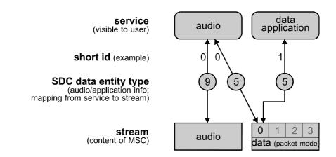
EXAMPLE 4: To make maximum use of the possibilities of a DRM multiplex, the following scenario is possible:
