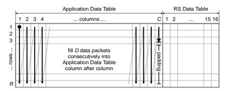
Figure 23: Placing data packets into FEC frame
