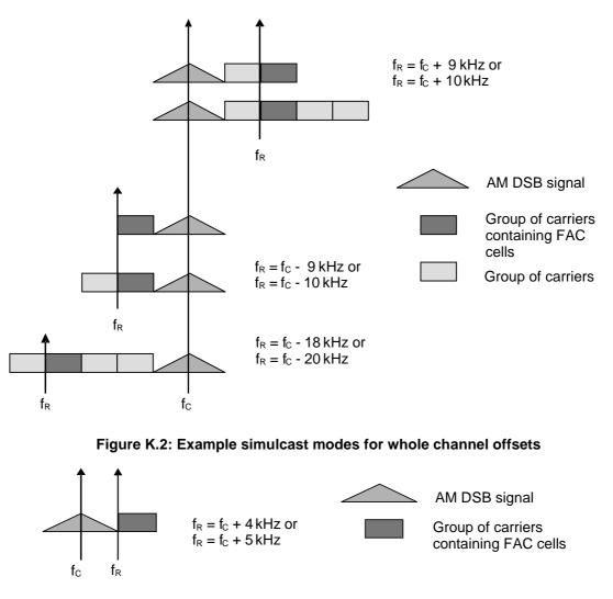
Figure K.3: Example simulcast modes for half channel offsets
