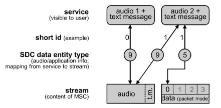
EXAMPLE 3: There is one audio service and one data service signalled to the user. The DRM multiplex consists of one audio stream and one data stream in packet mode containing one sub-stream. The data service points to the data application carried in the one sub-stream of the data stream. The audio service points to the audio stream and additionally also to the one sub-stream of the data stream.
