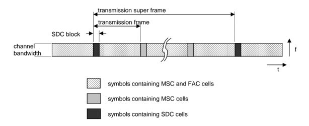
Figure 42: Time-frequency location of FAC and SDC signals
