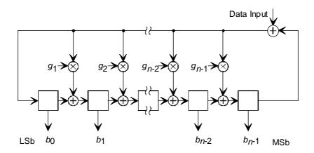
Figure D.1: General CRC block diagram
