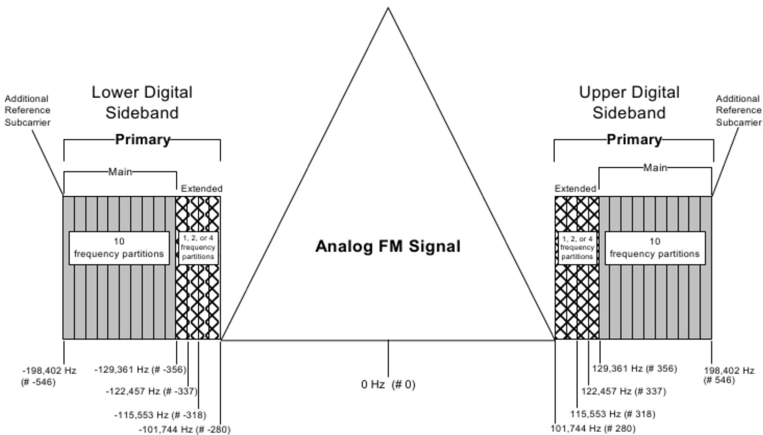
**Figure 7 Spectrum of the Extended Hybrid Waveform**
